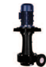
QHD Series (50/60 Hz) Max. flow: 2100L/min Max. head: 38m Main material: GFRPP/CFRPP/PVDF/CFRETFE Temperature range of liquid delivery: 0~80°C (GFRPP/CFRPP) 0~90°C (PVDF) 0~120°C (CFRETFE)
