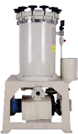
QH Series (50/60 Hz) Max. filtration capacity: 700L/min Main material: PPH/UPVC/CPVC/PVDF Temperature range of liquid delivery: 0~70℃ (PPH) 0~50℃ (UPVC) 0~60℃ (CPVC) 0~85℃ (PVDF) Customizable for larger filtration capacity
